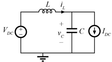
$$v_c(t) = V_{DC} + (V_0 - V_{DC}) \cos\left(\frac{t}{\sqrt{LC}}\right) + (I_0 - I_{DC}) \sqrt{\frac{L}{C}} \sin\left(\frac{t}{\sqrt{LC}}\right)$$
