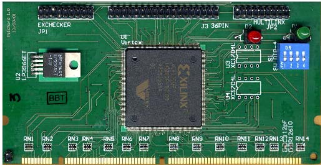
Figure 2.3 The Pilchard board
