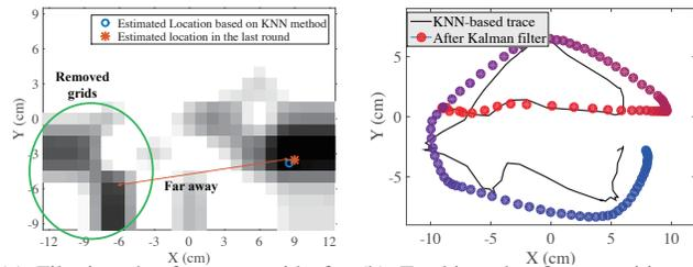
(a) Filtering the far-away grids for KNN-based localization (b) Tracking the finger writing of letter “e”
