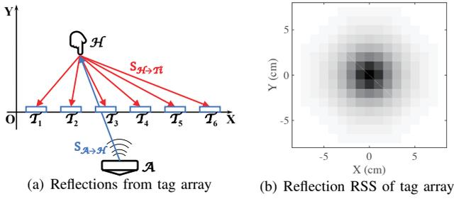
Fig. 5. Reflection model of a tag array.
