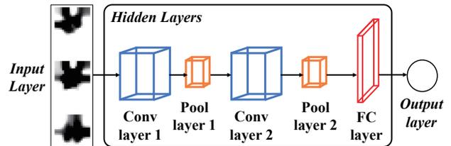
Fig. 12. Illustration of CNN structure for gesture recognition.
