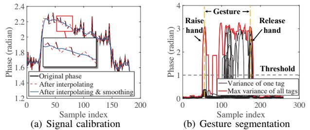
Fig. 8. Illustration of signal preprocessing in RF-finger.
