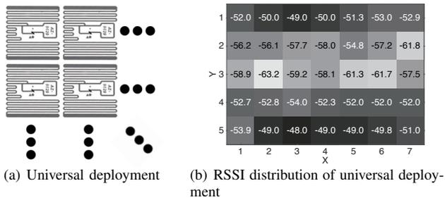
Fig. 3. Preliminary study of the tag array deployment.
