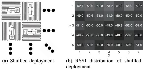
Fig. 7. Shuffled deployment of the dense tag array.
