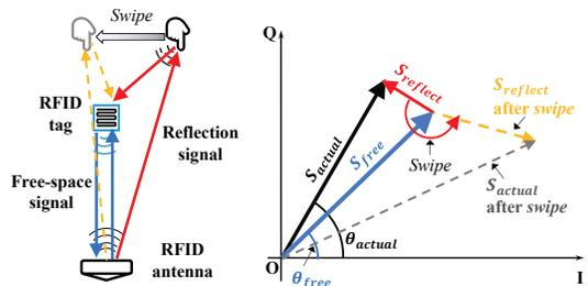
Fig. 4. Reflection model of a tag.
