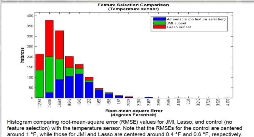
For each sensor, we trained 500 networks and calculated the root-mean-square-error between the network's output and the correct value. The following two figures present histograms of these results.
