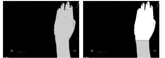
Figure 4. Image before and after bounding box is applied to the hand and Flood-Fill at the centroid to separate the arm from the hand
