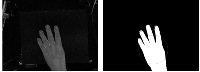
Figure 6. Original saturation channel and result after complete processing ; shows the arc swept out to count the fingers
