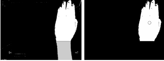
Figure 5. Image before and after threshold is applied to remove noise; the circle was added only to enhance the location of the refined centroid
