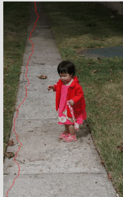
Figure 1: Seam Example: Optimal “slice” (red line) to find unimportant pixels to remove
