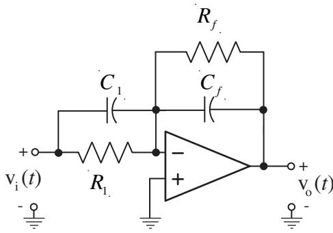
Let  $C_f = 1\text{nF}$ . Then  $C_1 = 5\text{nF}$ ,  $R_l = 20\text{ k}\Omega$  and  $R_f = 5\text{k}\Omega$ . (Complete except for the minus sign.)
