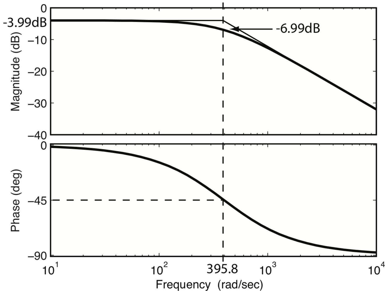
Let  $C_1 = 20 \text{ nF}$ ,  $R_1 = 20 \text{ k}\Omega$ ,  $C_2 = 100 \text{ nF}$ ,  $R_2 = 5 \text{ k}\Omega$  and  $K = 8$ .
