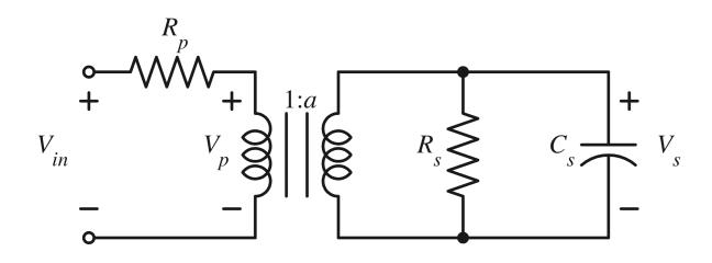
Let  $R_p = 2 \text{ k}\Omega$ , a = 4,  $R_s = 6 \text{ k}\Omega$ ,  $C_s = 500 \text{ nF}$
