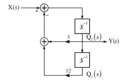
Let the responses of the integrators be the states  $Q_1(s)$  and  $Q_2(s)$  as indicated on the block diagram. Then
