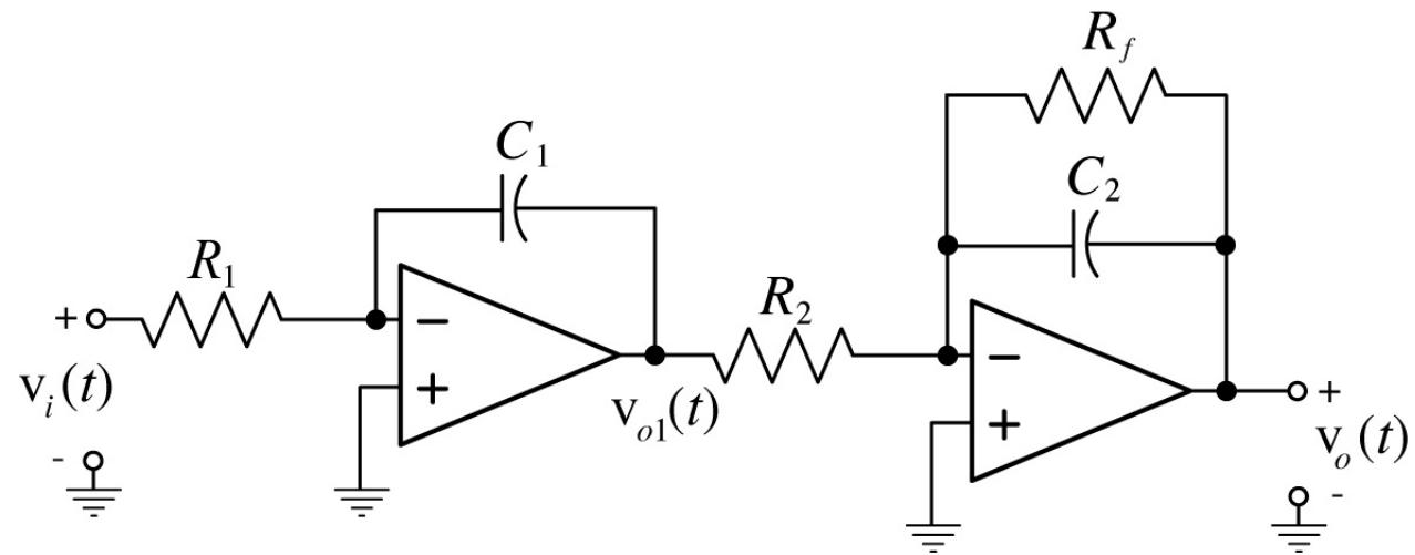
$$v_i(t)/R_1 = -C_1 v'_{o1}(t) , \quad v_{o1}(t)/R_2 = -C_2 v'_o(t) - v_o(t)/R_f$$
