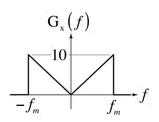
A message x(t), with W = 5kHz, DSB modulates a carrier of frequency  $f_c = 1$ MHz and amplitude  $A_c = 1$ . The channel loss is 20 dB. Nonwhite noise with power spectral density as shown in the figure below adds to the signal prior to detection with a synchronous demodulator. Find the signal-to-noise ratio  $(S/N)_D$  assuming that the power of the signal is 1 W.
