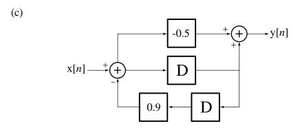
Designate the lower input to the last summer as w[n]. Then the excitation of the delay feeding that point is w[n+1] and
