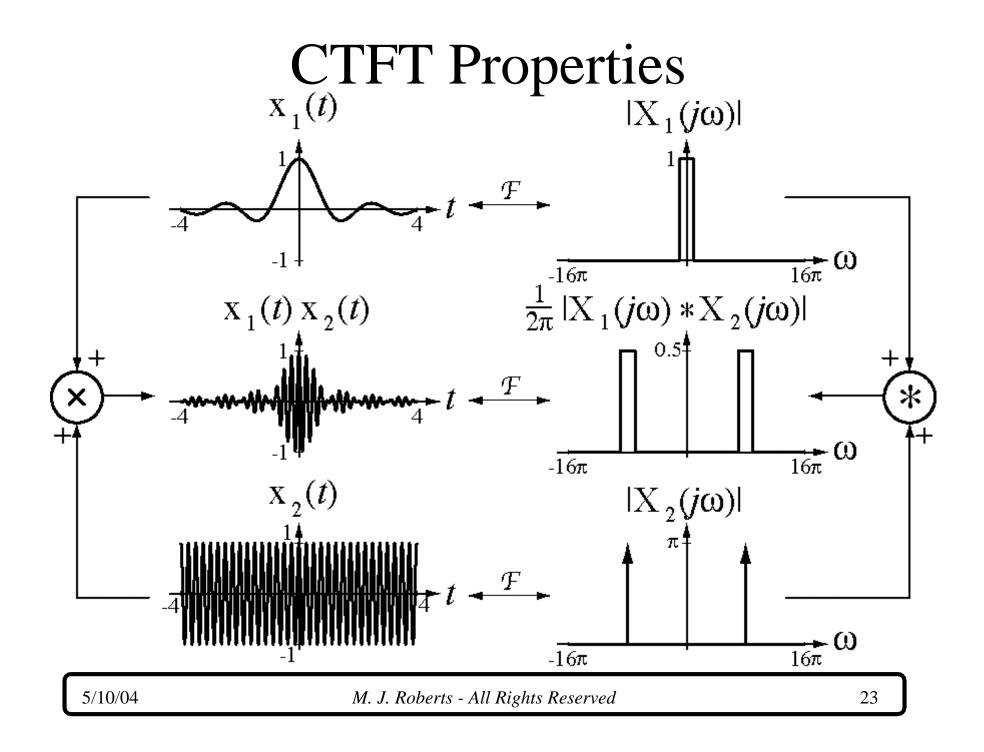
An important consequence of multiplication-convolution duality is the concept of the *transfer function*.
