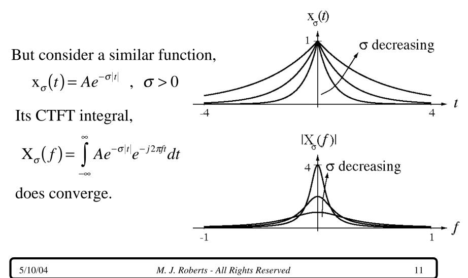
Convergence and the Generalized Fourier Transform Carrying out the integral,  $X_{\sigma}(f) = A \frac{2\sigma}{\sigma^2 + (2\pi f)^2}$ . Now let  $\sigma$  approach zero.
