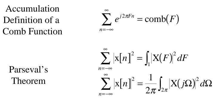
The signal energy is proportional to the integral of the squared magnitude of the DTFT of the signal over one period.
