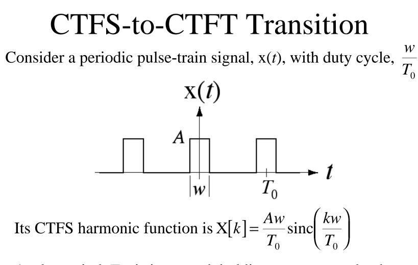
As the period,  $T_0$ , is increased, holding w constant, the duty cycle is decreased. When the period becomes infinite (and the duty cycle becomes zero) x(t) is no longer periodic.
