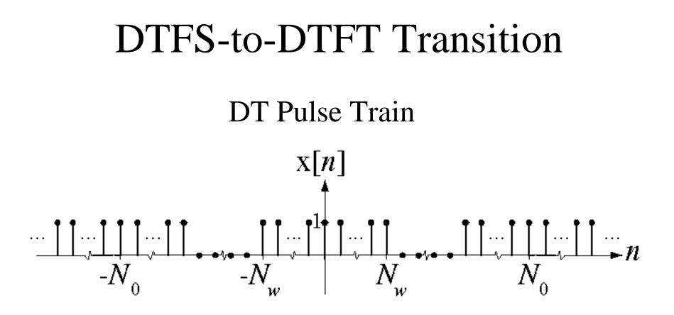
This DT periodic rectangular-wave signal is analogous to the CT periodic rectangular-wave signal used to illustrate the transition from the CTFS to the CTFT.
