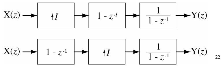
The transfer function of the cascaded integrator filter can be written as
