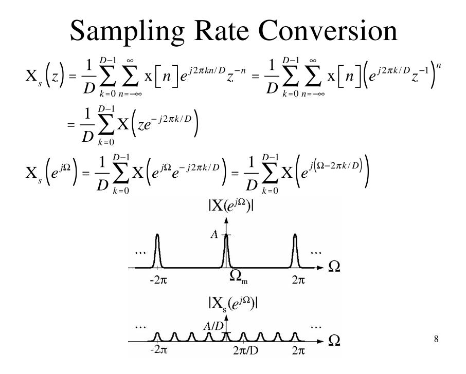
To reduce the number of samples, decimate the sampled signal to form  $x_d[n] = x_s[Dn]$ . The *z* transform of  $x_d[n]$  is
