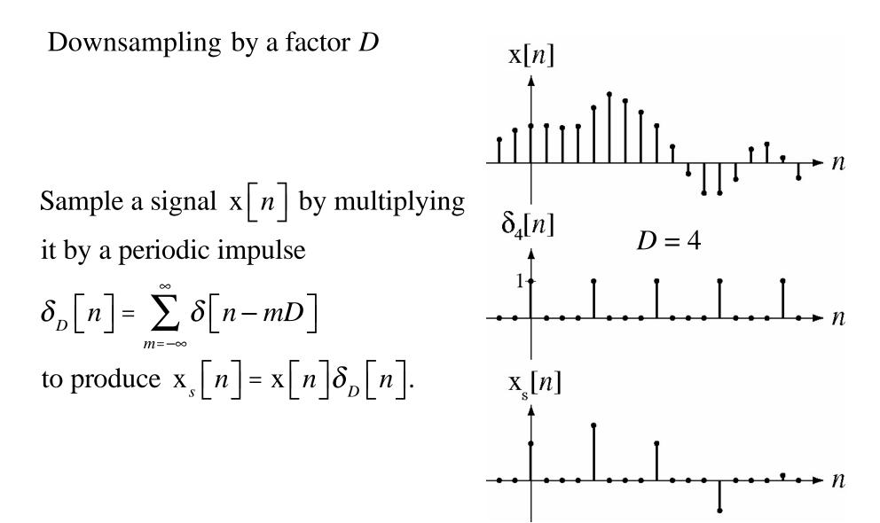
The discrete-time Fourier series harmonic function for  $\delta_D \lceil n \rceil$  is
