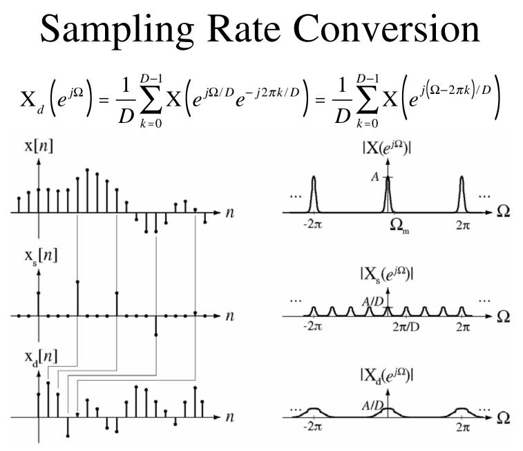
The opposite of downsampling is upsampling. If the original signal is  $x \lceil n \rceil$  the upsampled signal is
