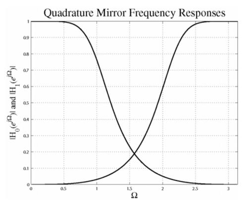
In summary, for elimination of aliases  $H_0(z) = H(z)$   $H_1(z) = H(-z)$   $G_0(z) = H(z)$   $G_1(z) = -H(-z)$
