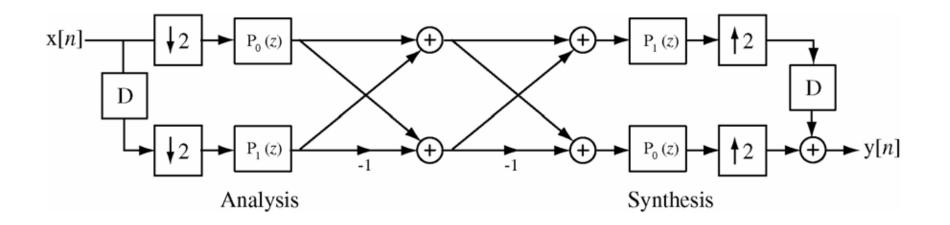
Perfect reconstruction of the input signal can be acheived by an FIR half-band filter of length 2N - 1. A half-band filter is a zero-phase FIR filter whose impulse response b[n] satisfies
