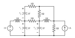
We can simplify the circuit for this problem by replacing all capacitors by open circuits and all inductors by short circuits. Also the upper-right hand resistor is shorted out and can be removed without changing any voltages or currents.
