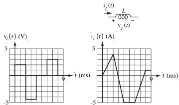
Between 0 and 2 ms the slope of the current is 2000 A/s. Therefore by  $v_L(t) = L\frac{d}{dt}(i_L(t))$ , the voltage is 2 volts.
