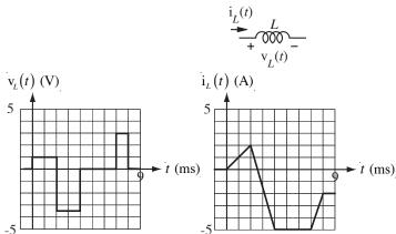
Between 0 and 2 ms the slope of the current is 1000 A/s. Therefore by  $v_L(t) = L\frac{d}{dt}(i_L(t))$ , the voltage is 1 volts.
