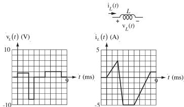
Between 0 and 2 ms the slope of the current is 1500 A/s. Therefore by  $v_L(t) = L\frac{d}{dt}(i_L(t))$ , the voltage is 1.5 volts.
