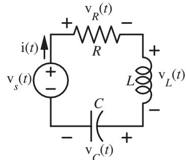
Before time  $t = 0$ ,  $v_s(t) = 6\text{V}$ ,  $i(t) = 0\text{A}$ ,  $v_L(t) = 0\text{V}$ ,  $v_C(t) = 6\text{V}$ ,  $v_R(t) = 0\text{V}$ .
