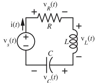
Before time  $t = 0$ ,  $v_s(t) = 3\text{V}$ ,  $i(t) = 0\text{A}$ ,  $v_L(t) = 0\text{V}$ ,  $v_C(t) = 3\text{V}$ ,  $v_R(t) = 0\text{V}$ .
