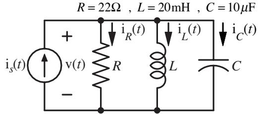
Before time  $t = 0$ ,  $i_s(t) = -2\text{A}$  ,  $v(t) = 0\text{V}$  ,  $i_L(t) = -2\text{A}$  ,  $i_C(t) = 0\text{A}$  ,  $i_R(t) = 0\text{A}$ .
