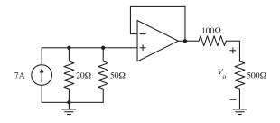
The operational amplifier is configured as a voltage follower with infinite input resistance and a voltage gain of +1. None of the source current can flow into the operational amplifier input and the voltage at that input is therefore
