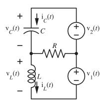
Before t = 0 all voltages and currents are constant, the capacitor is an open circuit and the inductor is a short circuit. There is no current through the capacitor and therefore no current anywhere in the circuit. By KVL around the top mesh the capacitor voltage must equal 5 V and that voltage will be the same at  $t = 0^+$ .
