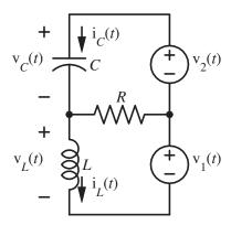
Before t = 0 all voltages and currents are constant, the capacitor is an open circuit and the inductor is a short circuit. There is no current through the capacitor and therefore no current anywhere in the circuit. By KVL around the top mesh the capacitor voltage must equal 15 V and that voltage will be the same at  $t = 0^+$ .
