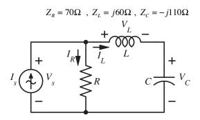
$$\begin{split} I_s &= I_R + I_L = 1.229 \angle -35.53^\circ \text{ A} \\ V_s &= V_L + V_C = -j50 = 50 \angle -90^\circ \text{ V} \\ \end{split} \quad V_L &= Z_L I_L = j60 = 60 \angle 90^\circ \text{ V} \\ V_C &= Z_C I_L = -j110 = 110 \angle -90^\circ \text{ V} \\ \end{split}$$
