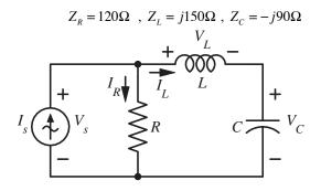
$$\begin{split} I_s &= I_R + I_L = 1.118 \angle 26.57^\circ \text{ A} & I_R &= V_s \ / \ R = 0.5 \angle 90^\circ \text{ A} \\ V_s &= V_L + V_C = j60 = 60 \angle 90^\circ \text{ V} & V_L = Z_L I_L = j150 = 150 \angle 90^\circ \text{ V} & V_C = Z_C I_L = -j90 = 90 \angle -90^\circ \text{ V} \end{split}$$
