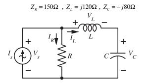
$$I_s = I_R + I_L = 1.035 \angle 14.93^{\circ} \text{ A} \qquad I_R = V_s / R = 0.2667 \angle 90^{\circ} \text{ A}$$
