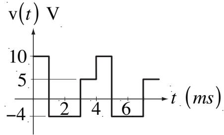
$$v_{avg} = \frac{10 \times 1 - 4 \times 2 + 5 \times 1}{4} = 7 / 4 = 1.75 \text{ V}$$
