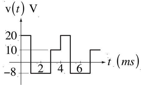
$$v_{avg} = \frac{20 \times 1 - 8 \times 2 + 10 \times 1}{4} = 14 / 4 = 3.5 \text{ V}$$
