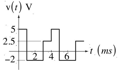
$$v_{avg} = \frac{5 \times 1 - 2 \times 2 + 2.5 \times 1}{4} = 7/8 = 0.875 \text{ V}$$
