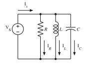
$$I_{R} = \frac{20\angle0^{\circ} \text{ V}}{2000\Omega} = 10\angle0^{\circ} \text{ mA}$$
