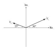
$V_2$  leads  $V_1$  by  $(180^{\circ} - 25^{\circ}) - 30^{\circ} = 125^{\circ} \Rightarrow V_1$  leads  $V_2$  by  $-125^{\circ}$
