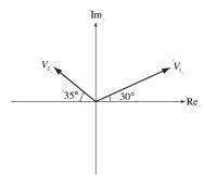
$V_2$  leads  $V_1$  by  $(180^{\circ} - 35^{\circ}) - 30^{\circ} = 115^{\circ} \Rightarrow V_1$  leads  $V_2$  by  $-115^{\circ}$
