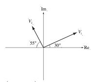
$V_2$  leads  $V_1$  by  $(180^\circ - 55^\circ) - 30^\circ = 95^\circ \Rightarrow V_1$  leads  $V_2$  by  $-95^\circ$
