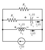
Before time t = 0 the capacitor current and the inductor voltage are both zero. All the current flows through the inductor. Therefore  $i_L(0^-) = i_s(0^-) = -6$ . Since there is no current flowing anywhere else at that time (and never has been) all the other currents and voltages are zero. So  $v_C(0^-) = 0$ .
