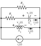
Before time t = 0 the capacitor current and the inductor voltage are both zero. All the current flows through the inductor. Therefore  $i_L(0^-) = i_s(0^-) = -4$ . Since there is no current flowing anywhere else at that time (and never has been) all the other currents and voltages are zero. So  $v_C(0^-) = 0$ .
