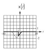
(a) In the space provided below draw a graph of  $x[n] = \{1 - ramp[2(n+2)]\}u[n-1]$  over the time range -10 < n < 10. On the graph put a vertical scale. The graph should be accurate enough to be able to read approximate function values from it.
