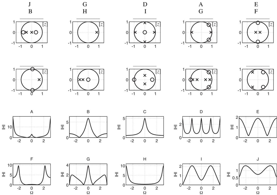
3. Match pole-zero diagrams to frequency responses by writing the letter designation of the magnitude frequency response that matches each pole-zero diagram in the blank space above that pole-zero diagram.
