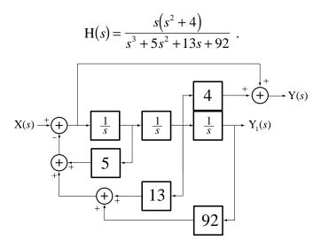
6. (10 pts) Draw a parallel system diagram of the system with the transfer function,
