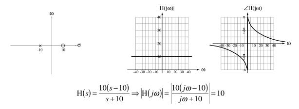
At any frequency the zero vector and the pole vector are always the same length so the transfer function magnitude is constant.
