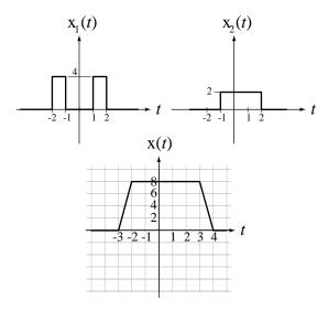
36. A linear system has an excitation, x(t), and a response, y(t). It is characterized by its impulse response,  $h(t) = 10 \operatorname{sinc} \left[ 10^7 \left( t - 10^{-6} \right) \right]$ . Find a real, time-domain expression for the system response, y(t), if the system excitation is
