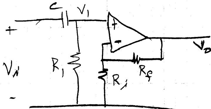
$$V_1 = \frac{R_i}{R_i + \frac{1}{sC}} = \frac{sR_i C}{1 + sR_i C} \frac{V_i}{}$$
