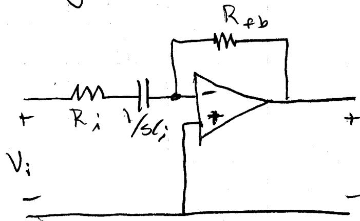
$$\frac{V_{o(s)}}{V_{i(s)}} = - \left[ \frac{R_{fb}}{R_i + \frac{1}{sC_i}} \right] = - \frac{s R_{fb} C_i}{1 + s R_i C_i}$$
