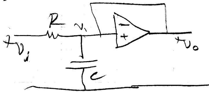
$$V_1 = -\frac{(1/sC) V_i}{R + 1/sC} = \frac{V_i}{1 + sRC}$$
