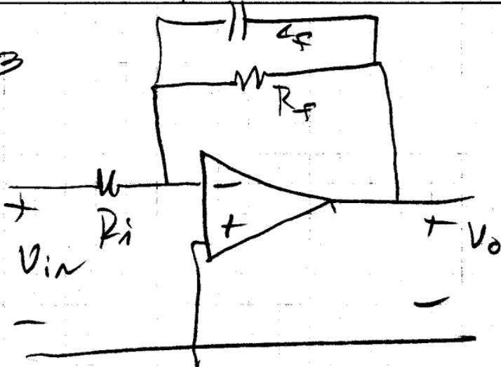
$$\frac{V_o}{V_{in}} = \frac{\frac{R_f / sC_f}{R_f + 1/sC_f}}{R_i}$$
