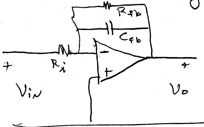
$$Z_{fb} = R_{fb} \parallel \frac{1}{sC_{fb}} = \frac{\frac{R_{fb}}{sC_{fb}}}{R_{fb} + \frac{1}{sC_{fb}}} = \frac{R_{fb}}{1 + sR_{fb}C_{fb}}$$
